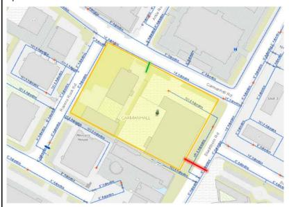
Separate storm and foul water connection services have to be provided for the Development. The surface and storm water from the site must be discharged only into an existing storm water network that does not discharge to an IW combined/foul sewer. The connection arrangement should be agreed with the Local Authority Drainage Division.
